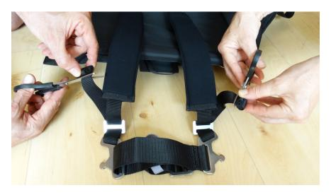
In order to take your current chest strap off your harness, you will first need to slide the leg straps out of the adjustment buckles that connect them to the chest strap. Since the blocking stitches at the end of the leg strap webbing do not allow you to do so, first you must cut the two ends as shown in the picture. Try to cut as precisely as possible because this will help you burning the cut edges properly, which is the following step.
