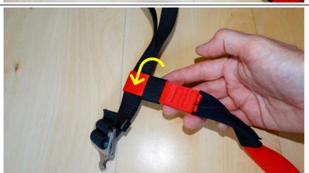
BEND THE LONG VELCRO BIT OVER the short one so that the leg strap is HELD FIRMLY at the very END OF THE new safe-T strap LOOP.
