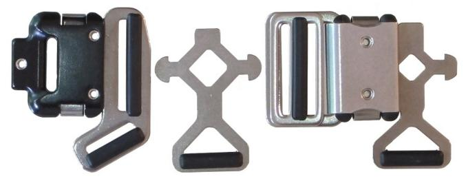
In the past three months, there have been two incidents involving older paraglider harnesses equipped with CLICK-LOCK buckles (HSi10) in the chest strap. The buckles had opened unintentionally during flight while they were under load. In one of the cases this happened during a SAT maneuver (spreading of the chest strap due to the pilot resting on the riser), in the other case the reason was presumably the load applied by the body weight of the pilot who was hanging only in the leg straps.
