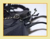
The speed system length is to be adjusted at the part where the strings are fixed to the bar itself.
