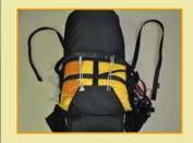
6) Using the strings from the handy kit, start closing the flaps of the container (strings are delivered in the handy kit).
