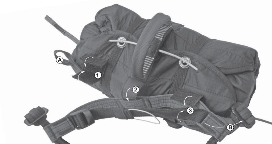
Pilot's view: Front container mounted correctly
