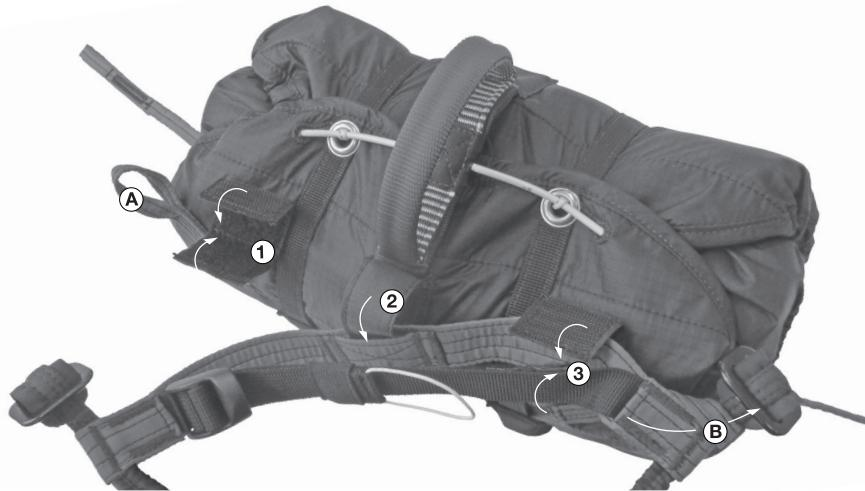
Pilot's view: Front container mounted correctly
